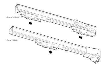
**Stack back:** When the master carrier reaches the fully open position it will stop (yellow LED4 is on). Now the open limit setting can be adjusted by hand, by remote or dry contact input. When the master carrier is not moved for 10 seconds, the yellow LED4 will go off and the open limit is set. The minimal automatic adjustment is 3 cm (1.2").
